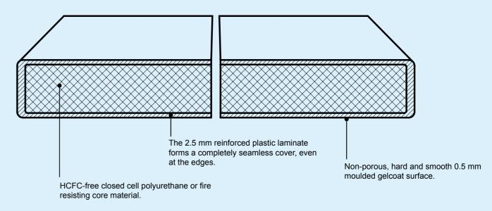
LAMI doors are manufactured using a pressure moulding process. This process produces a door leaf that is completely seamless and has no joints or lippings.
