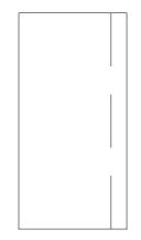
The doorleaf width can be reduced at the factory to any requested dimension. Cut edges are finished to their original standard with no visible seam.
