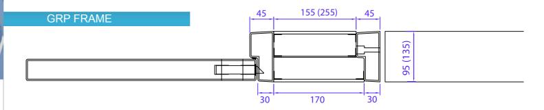
Traditional electric cable consoles available for aluminium frames and GRP frames.
