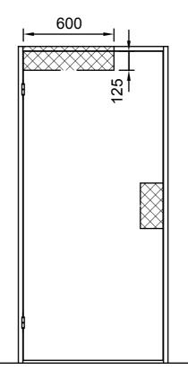
It is possible to include a reinforcement for a pull handle or door automation device or other ironmongery within the door leaf in order to enable a proper installation. The reinforcements are placed accordint to customer's choice/design.
