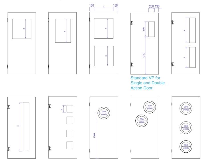
Maximum Vision Panel Sizes: (Not applicable to Fire Rated, Acoustic or X-ray Doors):
